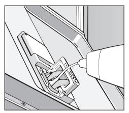
Close the dishwasher door halfway and pour liquid rinse aid into the storage container until it is visible on the surface of the screen. Do not add aid until the "Rinse aid" indicator lamp comes on.
